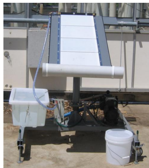
Figure 1: (a) schematic diagram and (b) photograph of the thin-film fixed-bed reactor (TFFBR) used in this study.
